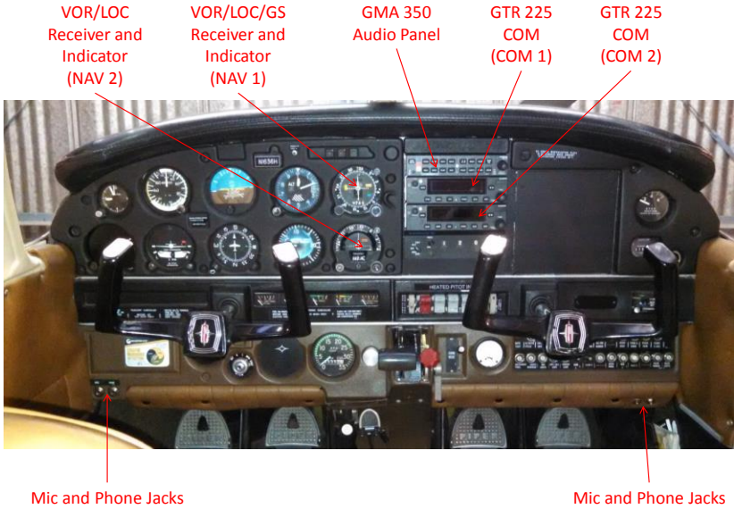
Figure 1: Avionics in N1636H
