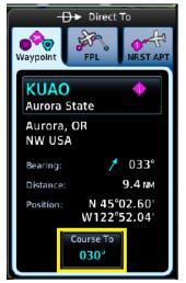
To use this feature, it starts out just like inputting a direct-to. the Direct-To button, choose your waypoint, and then hit the "Course To" button highlighted in the figure. This will open up a window that allows you to type in a desired course, such as shown of 030° when the direct to is actually 033°.
