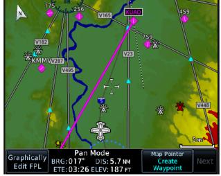
For marginal VFR flights when cleared straight-in, you can set this number to be the runway heading, which will get you close to lined up with the runway from farther away. When dealing with the smoke during the summer months, sometimes this feature can be very useful to help find a runway when around the haze. For the holds, this can then for your inbound leg of the unpublished hold, providing navigation guidance on any hold point for at least the inbound leg.
